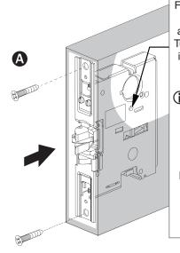
For TP, K and L trims with outside cylinder to lock and unlock trim function: Turn set screw all the way in until screw head is no longer visible.
