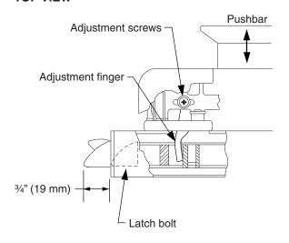
Loosen adjustment screws and adjust finger in or out until latch bolt is fully retracted (with pushbar down) and fully extended 34" (with pushbar up).
