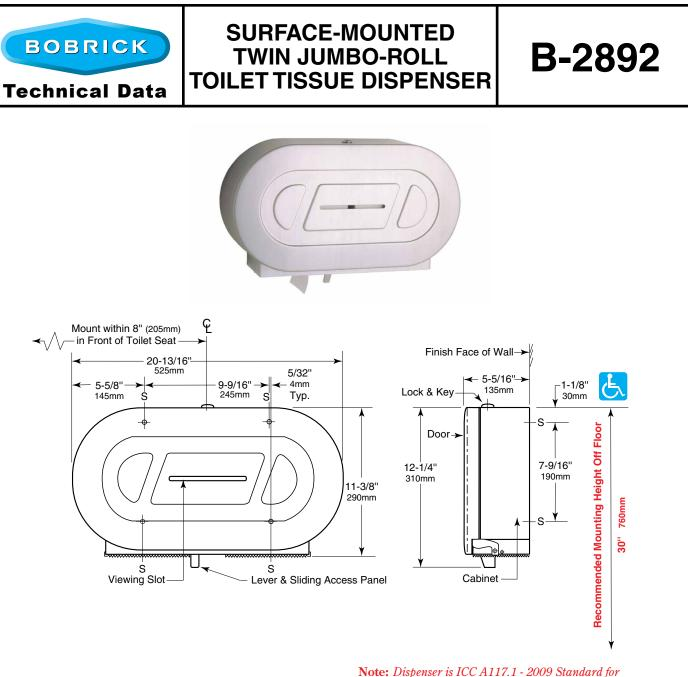
**Note:** Dispenser is ICC A117.1 - 2009 Standard for Accessibility compliant. Unit can be located below grab bar, in area 24" minimum to 42" maximum from rear wall, with outlet 18" minimum above floor.
