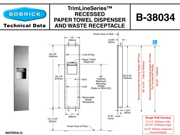
Cabinet — 18-8, Type-304, heavy-gauge stainless steel. All-welded construction.
