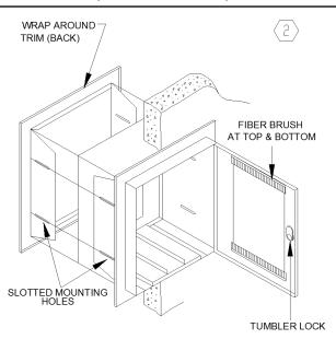
MOUNT AND ADJUST WRAP AROUND BACK TRIM TO WALL THICKNESS
