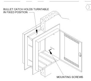
SECURE TO WALL WITH MOUNTING SCREWS THRU SLOTTED HOLES
