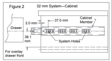
Use only the 32 mm system holes or the wood screw holes located at the tip of the breathing tabs. Do not use any other holes on the cabinet member for mounting (Figure 3).
